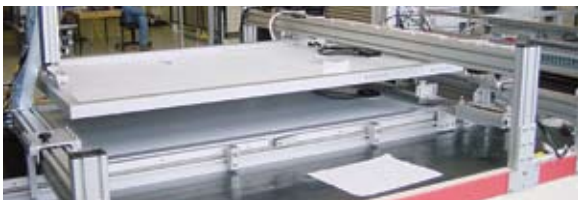
Evergreen Solar power tester with a calibrated solar panel mounted on top
