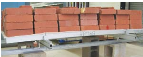
Snow load testing of Evergreen Solar panels at Arizona State University, USA
